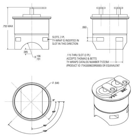
ORIENTATION OF TUBE ANGLE IS SHOWN ABOVE AT 90-DEGREES
