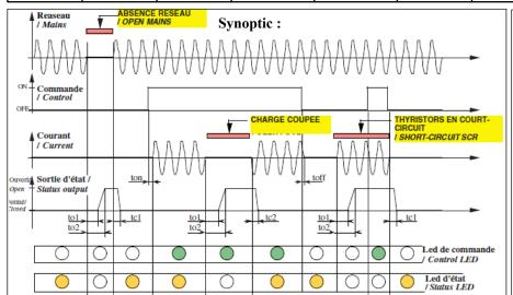
\* Status (static output) is normally closed without failure on the relay and the load, and the yellow LED is switched ON:
