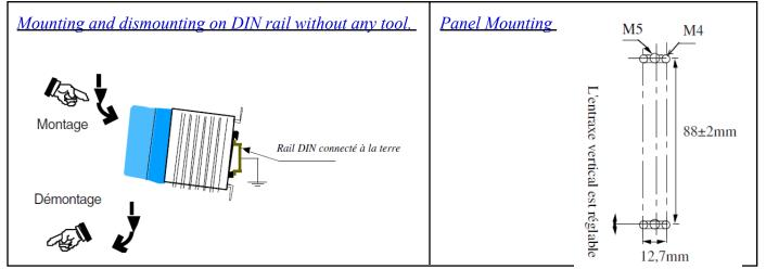
Warning! semiconductor relays don't provide any galvanic insulation between the load and the mains. Always use in conjunction with an adapted circuit breaker with isolation feature or a similar device in order to ensure a reliable isolation in the event of wrong function and when the relay must be insulated from the mains (maintenance; if not used for a long duration ...).
